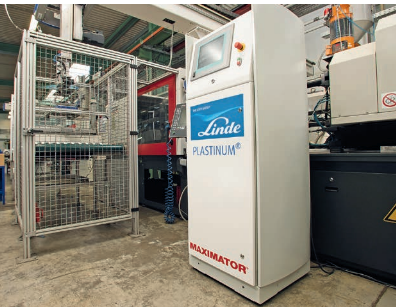
Fig. 6. The pressure control module (Linde) has to respond quickly and keep the counter-pressure constant to the end of the flow path by releasing gas as the melt flows in (© Linde)
