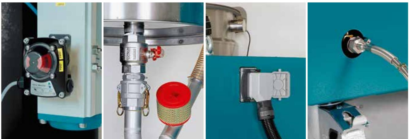
Left: Pressure conveying shut-off valve on the impregnating unit
