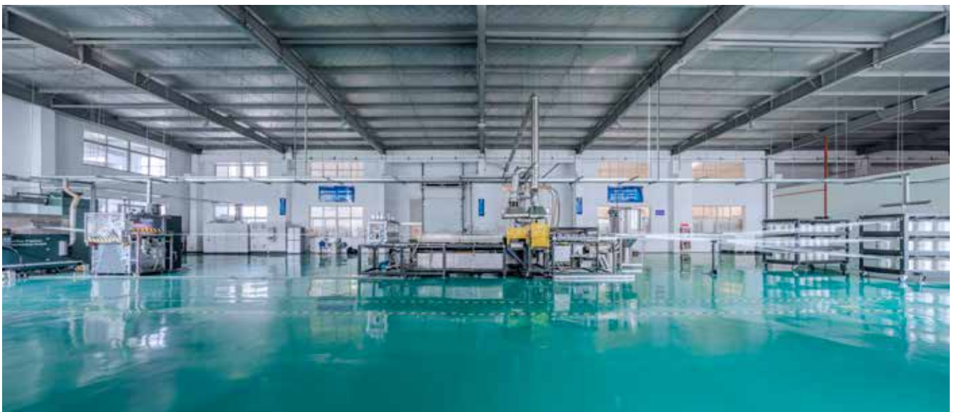
The LFT pultrusion line is approx. 30 m long and was adapted to the space available at Chinese plastics processor HCJH.
